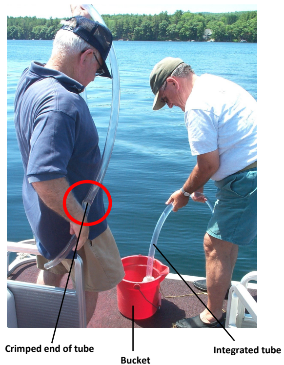
Figure 8. Using the Integrate Tube
