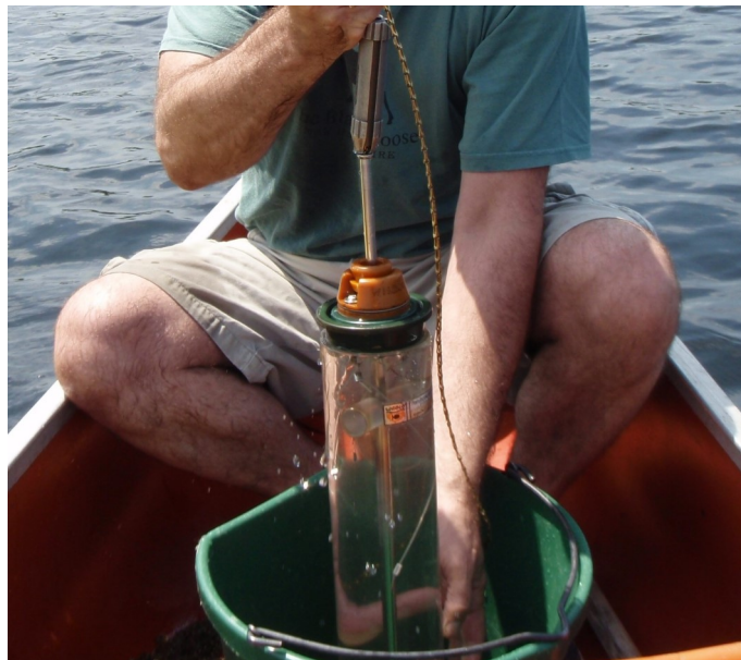
Method 1: Compositing with a Kemmerer bottle and bucket
