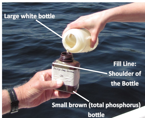
Figure 4. Total Phosphorus Bottle Filling
