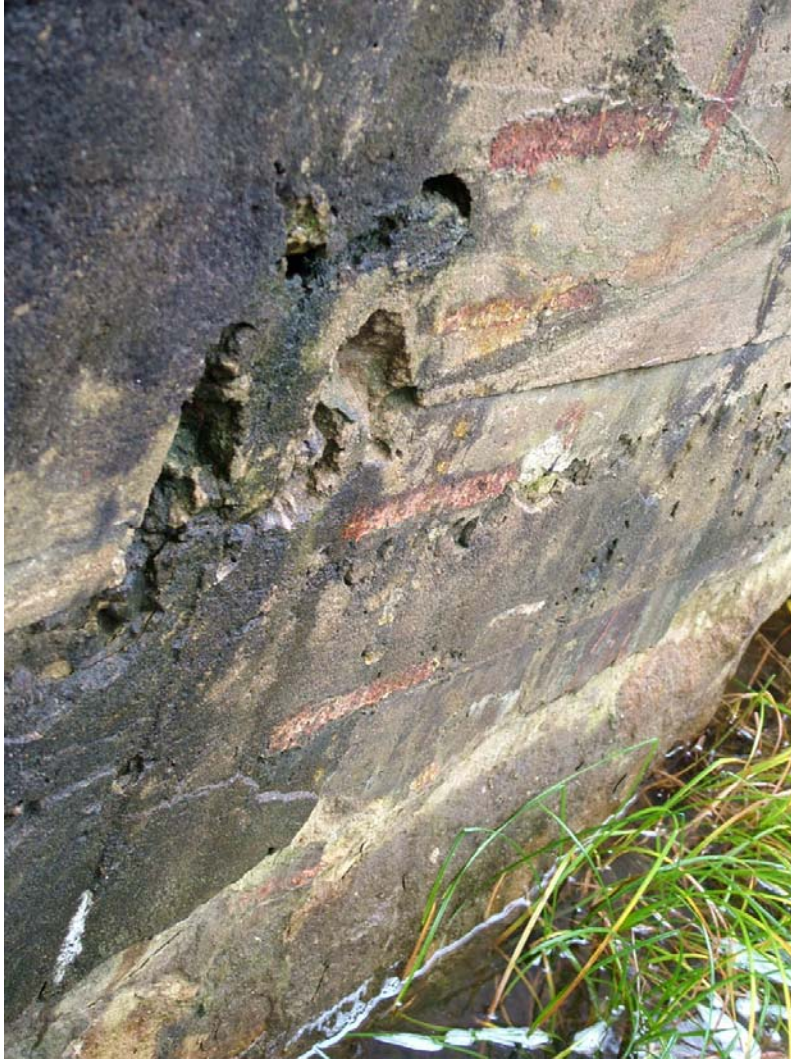
Figure 3. Hand painted gage at the shorebank fishing access on the Upper Souhegan River in Greenville, New Hampshire.
