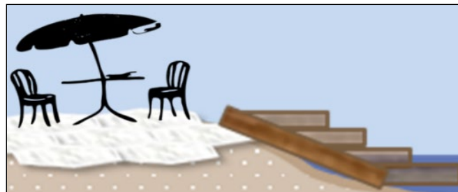
Figure 4 - Access stairs to and from water access structures. Steps made from stone, concrete or similar materials may be incorporated in the design of a water access structures, but they must not exceed six feet in width.
